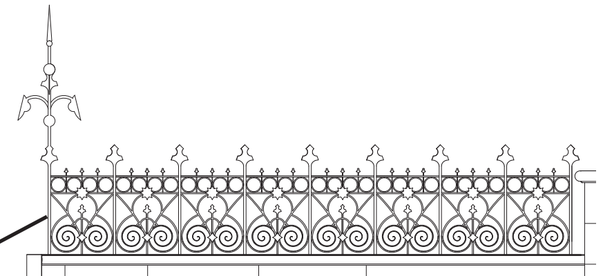
2 DETAIL OF TYPICAL NEW ROOF CRESTING AND FINIAL 3/8" = 1'-0"
