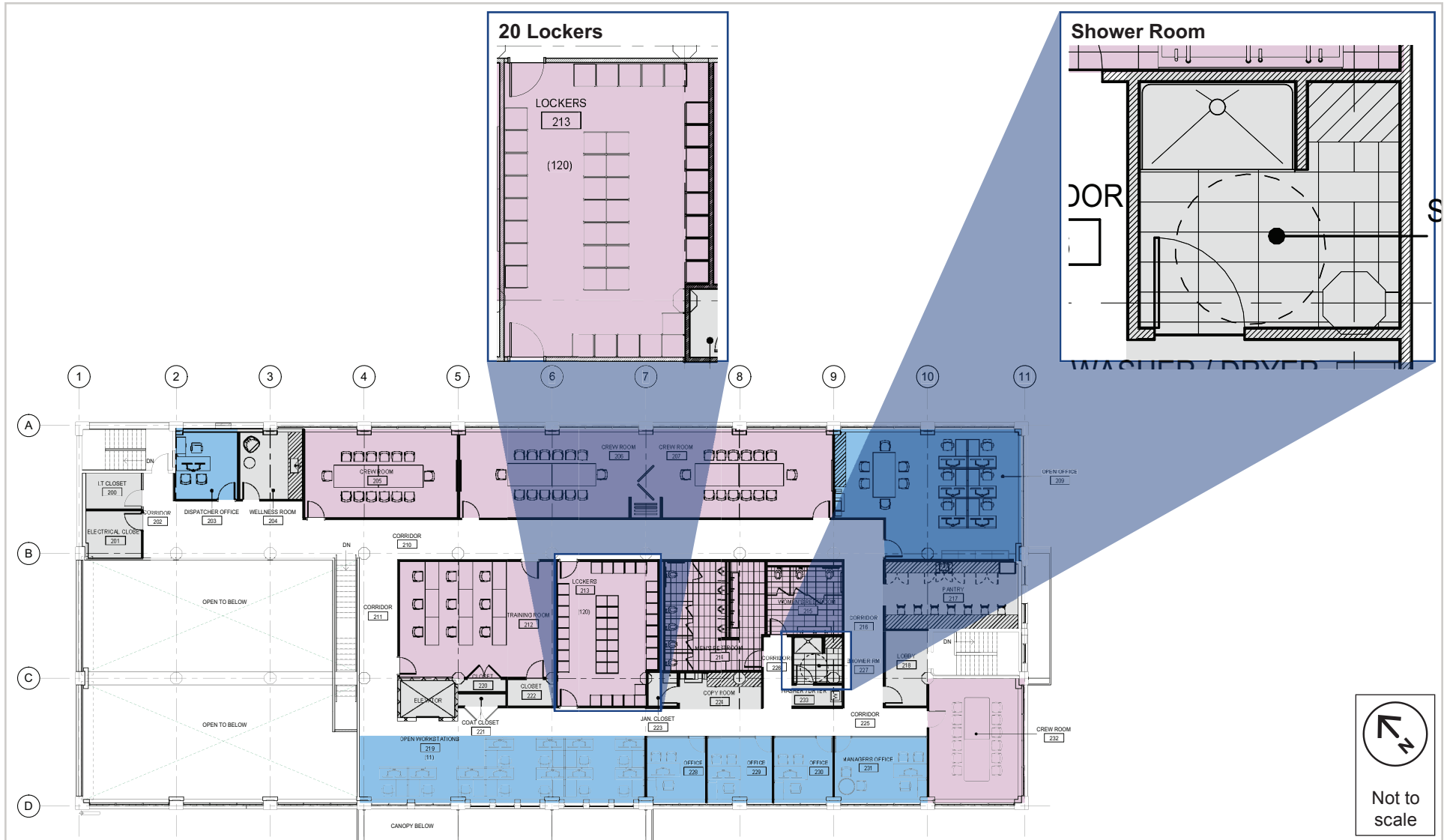
Figure 9. Internal Second Floor Plan: Lockers and Showers
