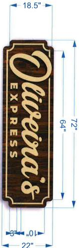
**Material:**High-density, rigid polyurethane foam (HDU), 15 lb per ft³ density
