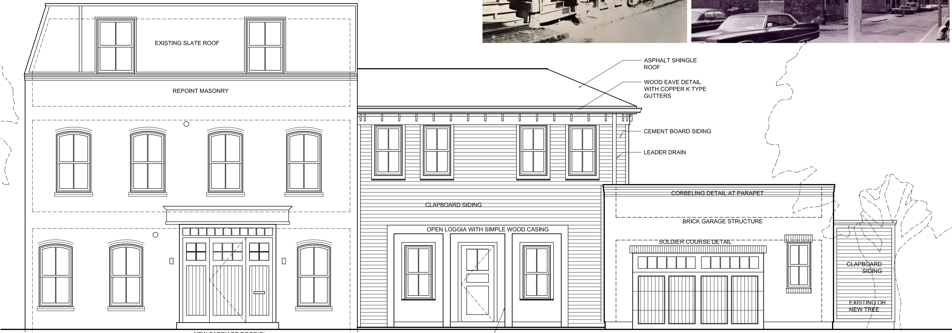
1 WEST ELEVATION (BRADFORD STREET) 1/4"=1'-0"
