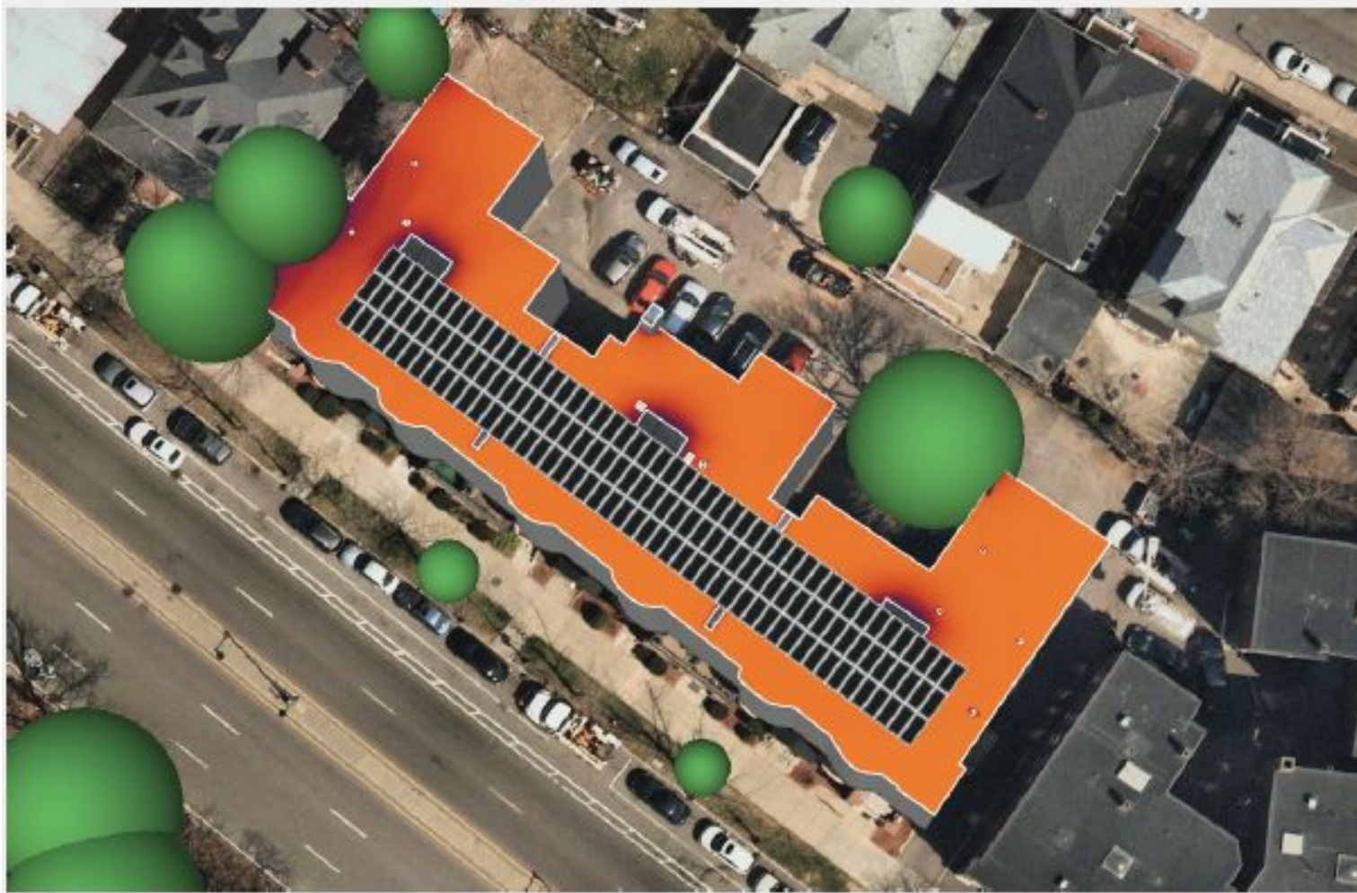
Solar Layout (70.6 kW, Tier 1, 490 Watt Panels)
