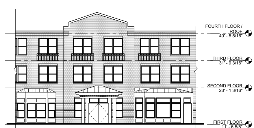
7A ELEVATION 7 - EXISTING 1/8" = 1'-0"
