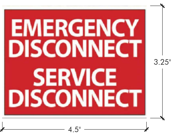
A PROPOSED "EMERGENCY DISCONNECT" PLACARD
