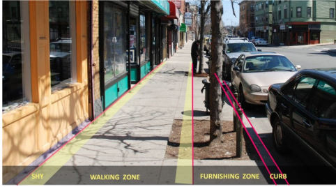
The sidewalk is comprised of a number of zones. People tend to shy away from walking next to buildings and other edges and, where there is inadequate width, people walk everywhere.
