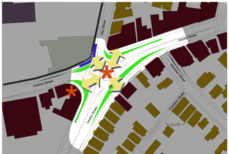
The concept to remedy this situation is to reduce the amount of roadway by widening the sidewalks. The widening of the sidewalks creates more room for pedestrians and streetscape amenities to support a walking environment. It also significantly reduces the length of the crosswalks which increase pedestrian safety.
