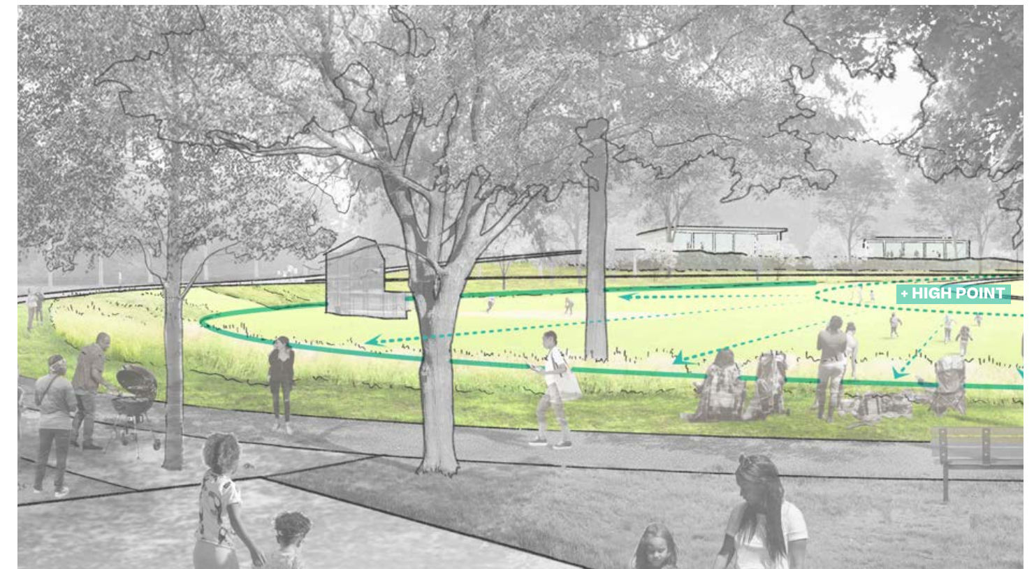
The proposed Playstead incorporates design features that improve both stormwater management and plant diversity. By regrading the fields with a central high point, surface runoff flows towards a grassland embankment with a french drain at its base to capture water at the edges.
