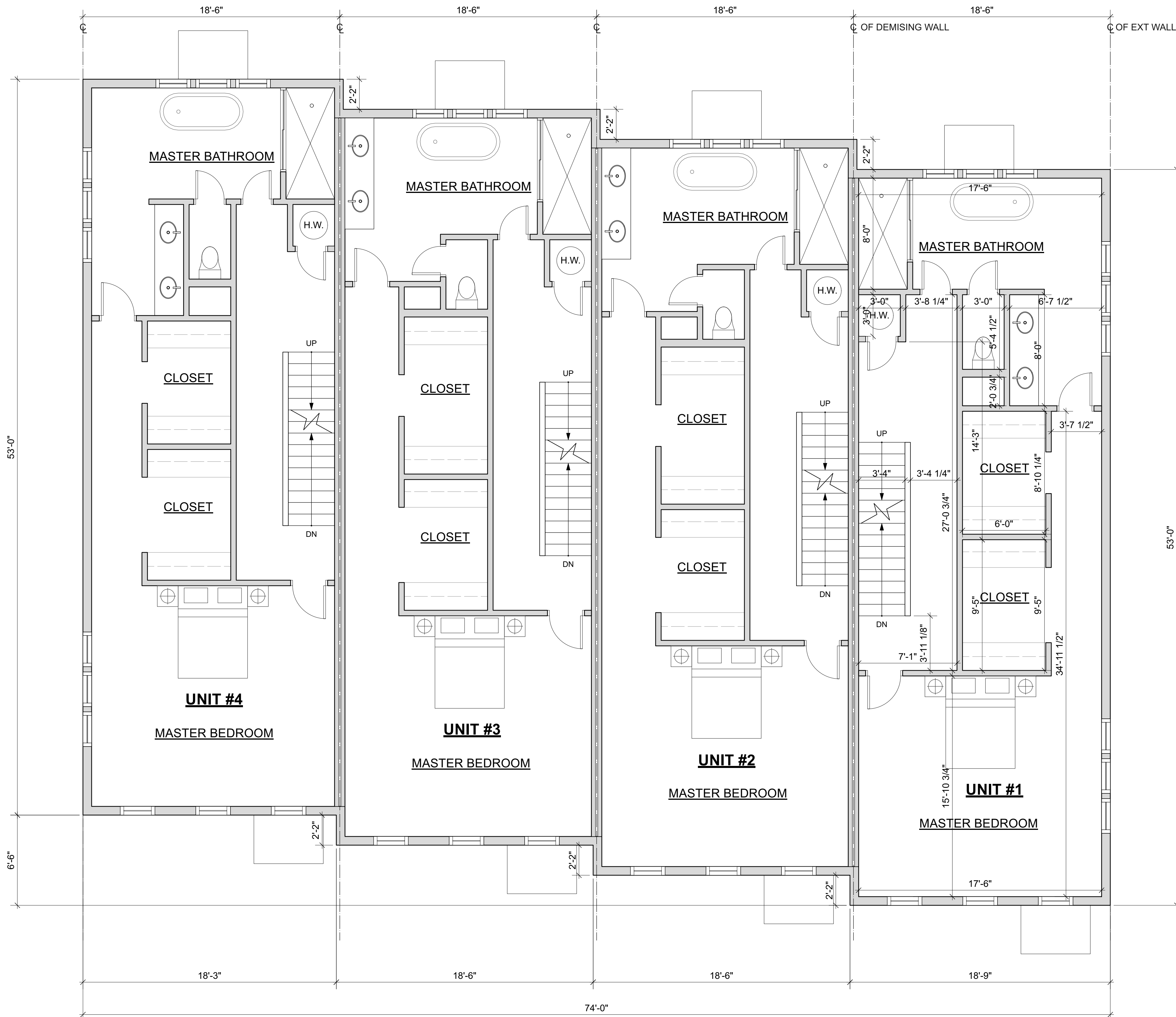
1 PROPOSED SECOND FLOOR PLAN Scale: 1/4" = 1'-0"
