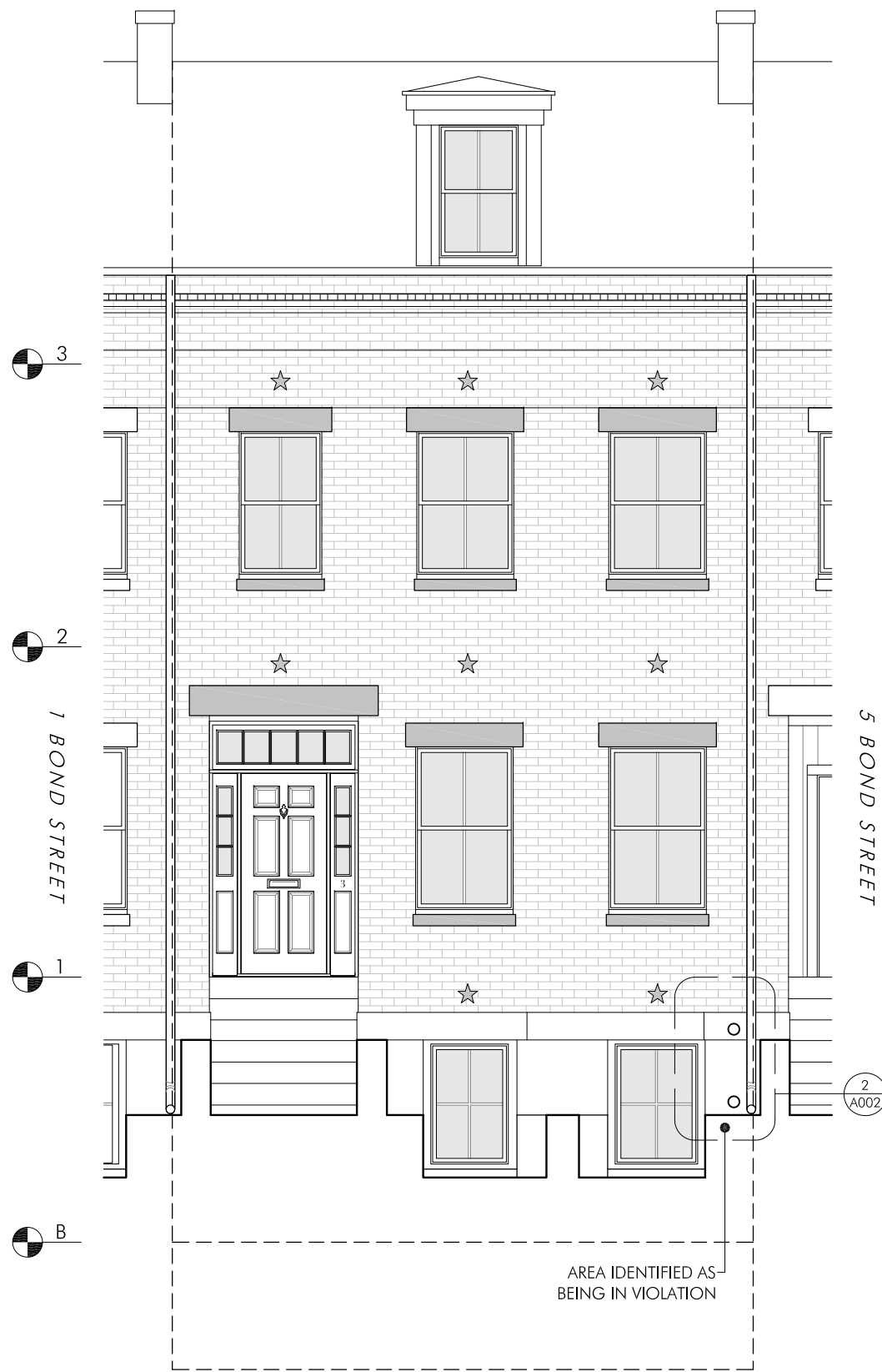
1 EXISTING EXTERIOR ELEVATION - FRONT SCALE: 3/16" = 1'-0"
