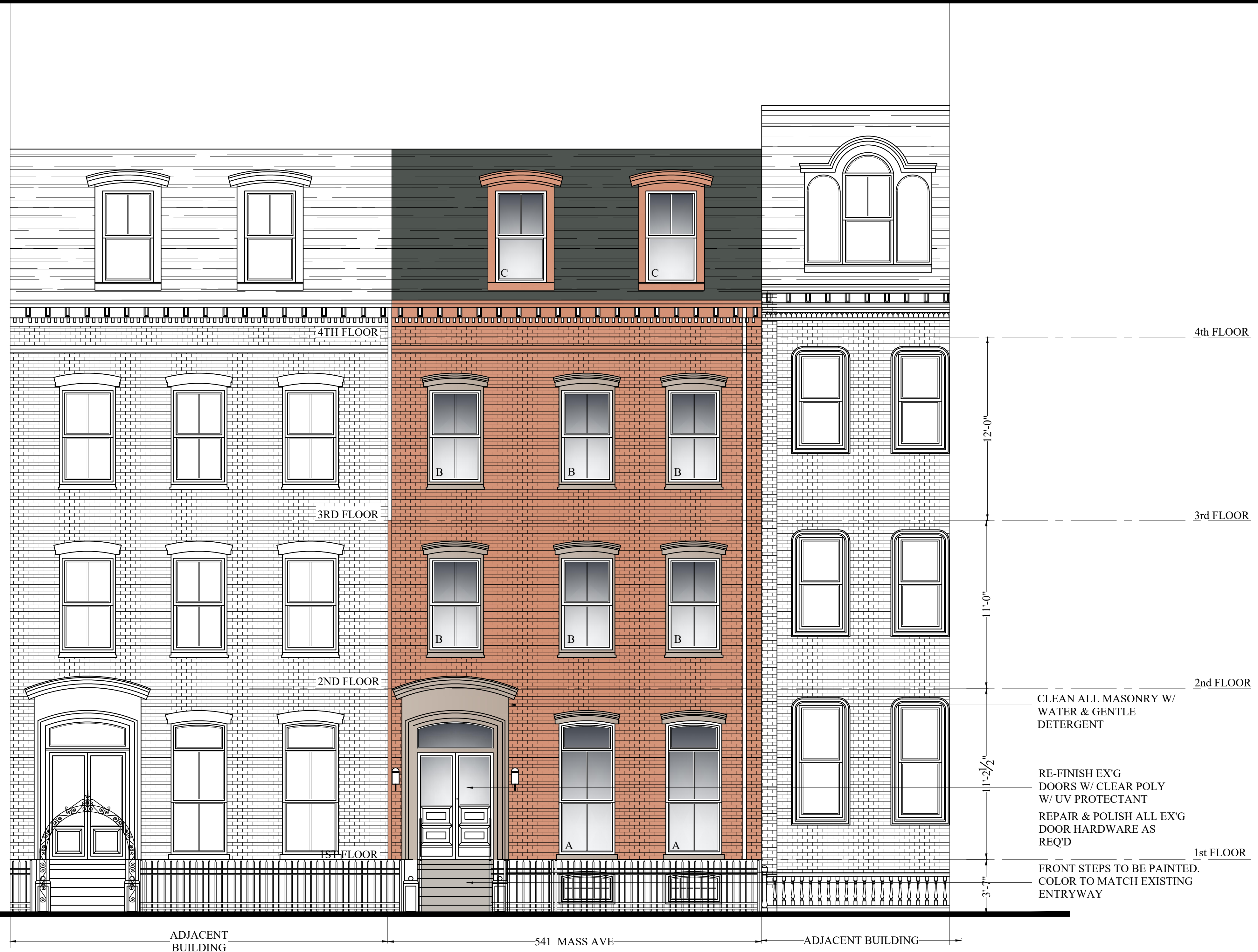
PROPOSED FRONT ( MASSACHUSETTS AVE ) ELEVATION 1/4" = 1'-0"
