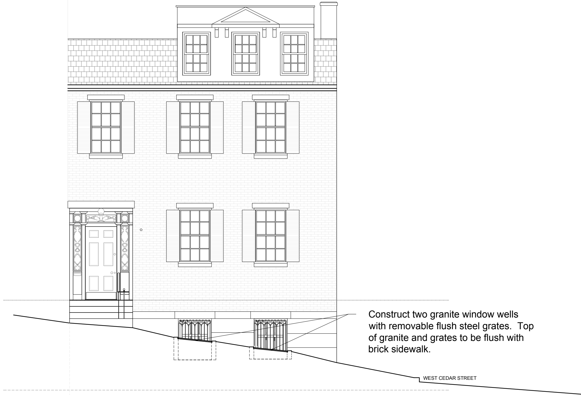
104 MT VERNON, NORTH ELEVATION 3/16" = 1'-0"
