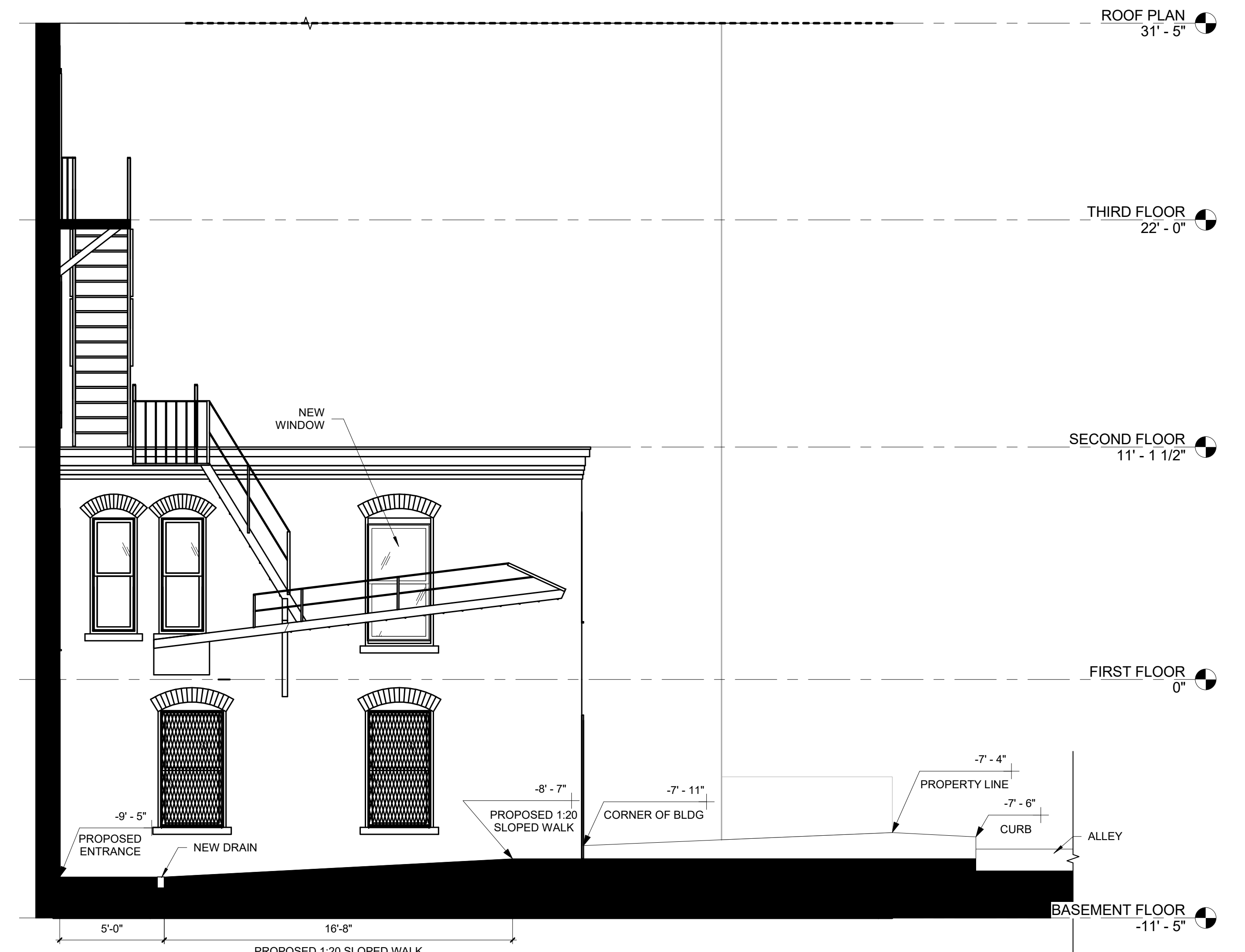
2 NORTH EAST ELEVATION - NEW CONSTRUCTION 1/4" = 1'-0"
