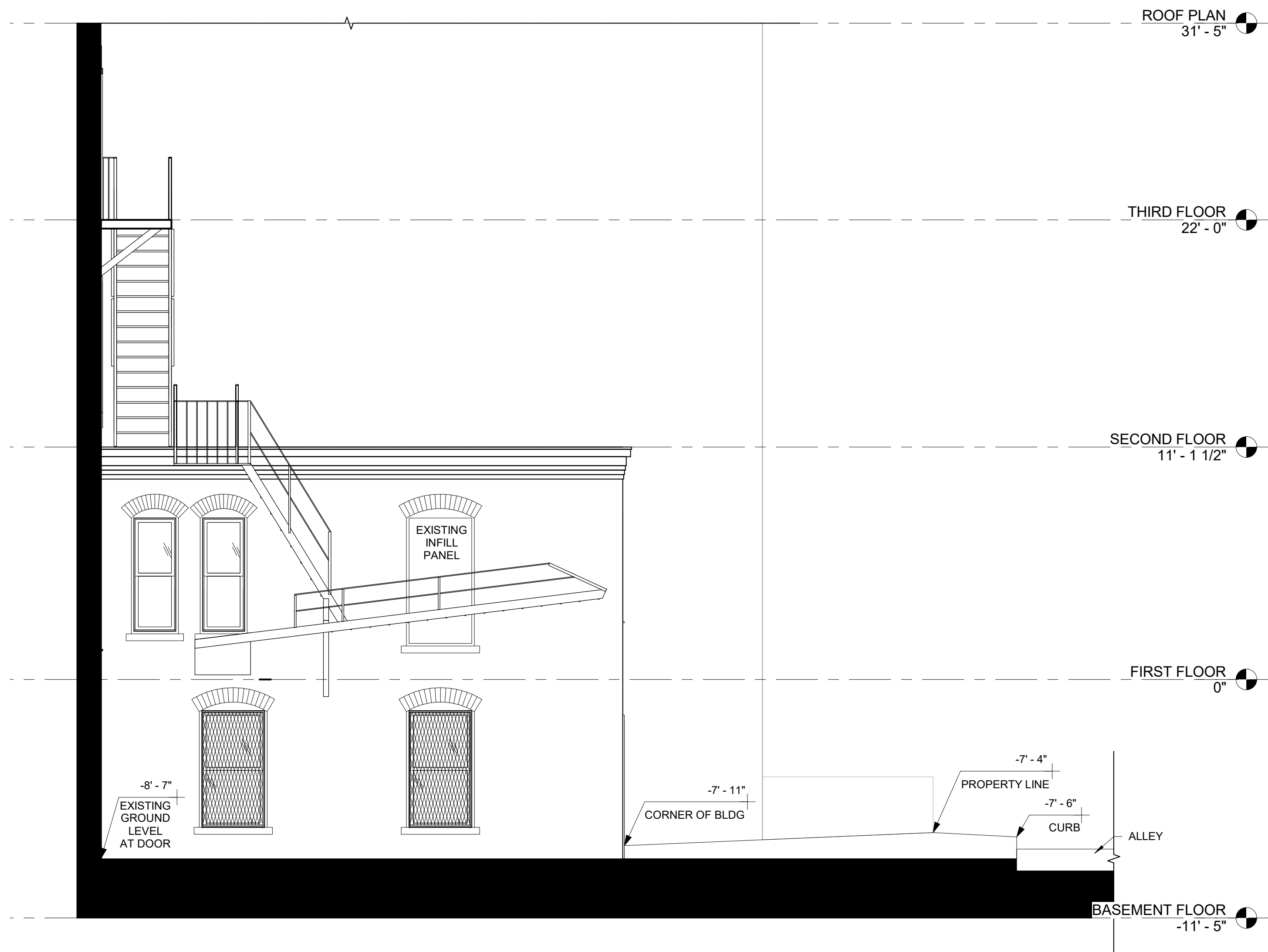
1 NORTH EAST ELEVATION - EXISTING 1/4" = 1'-0"
