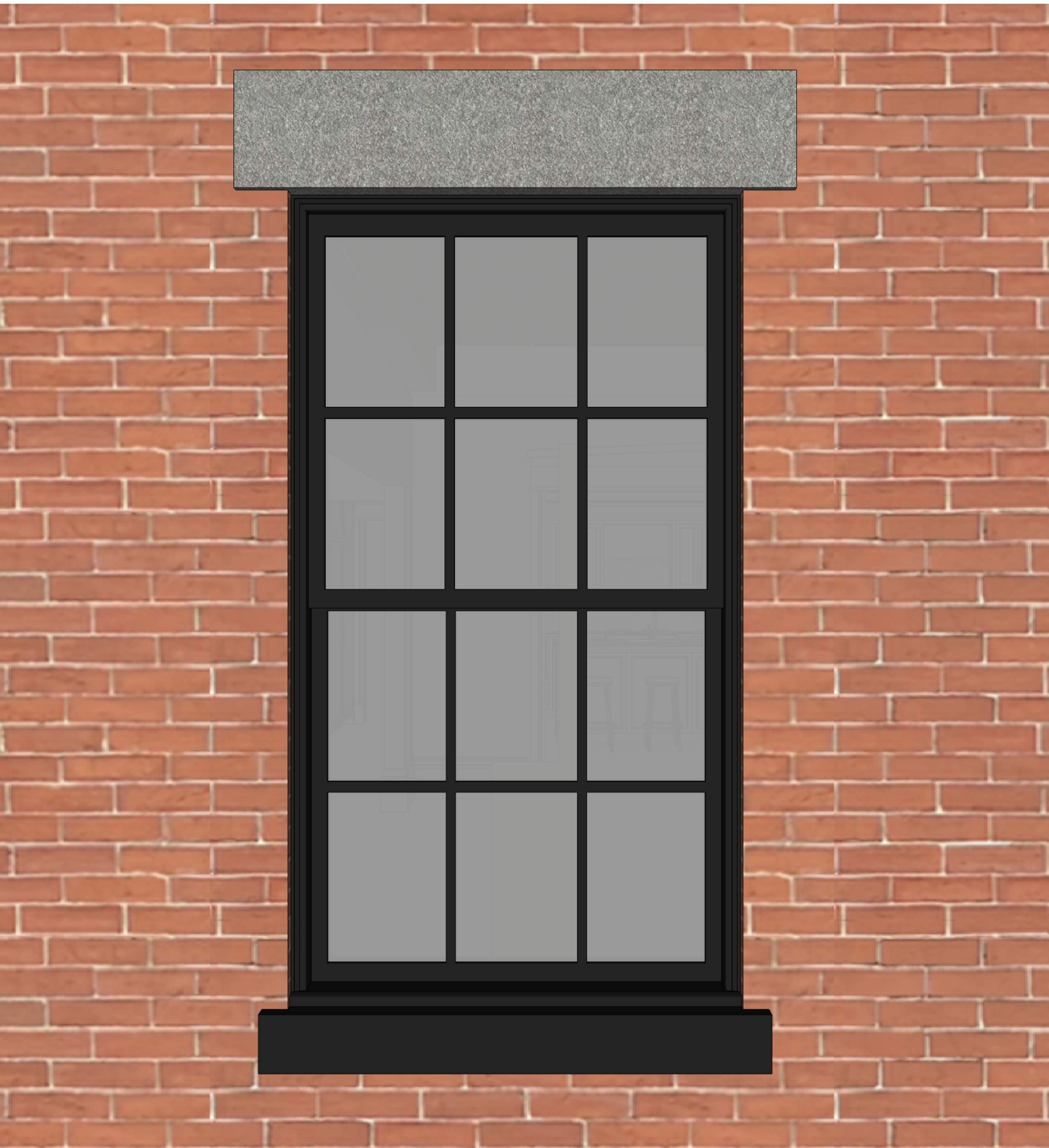
TYPICAL, REPLACEMENT DOUBLE-HUNG WINDOW WITHOUT SHUTTER
