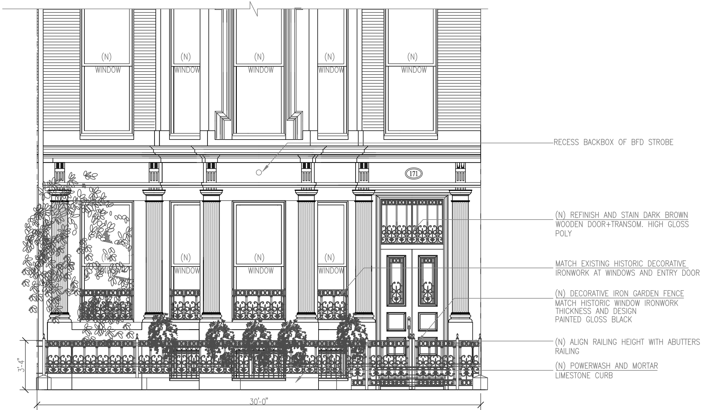
1 PROPOSED FRONT YARD ELEVATION SCALE: 1/4" = 1'-0"
